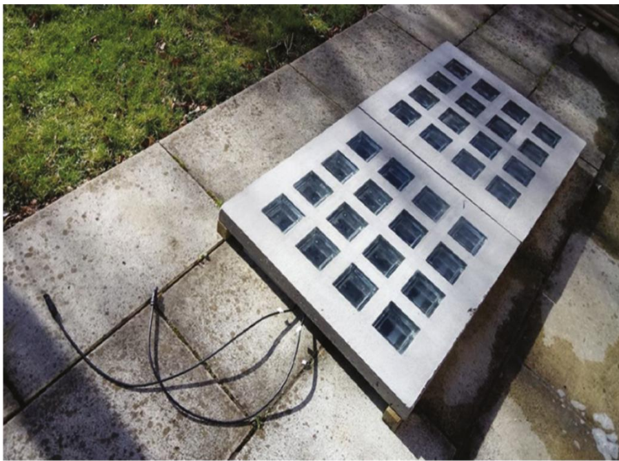
This prototype of a solar powered sidewalk paver is an emerging technology that will revolutionize urban planning. Photo credit: Paving the Sidewalks With Solar , April 30, 2018.
